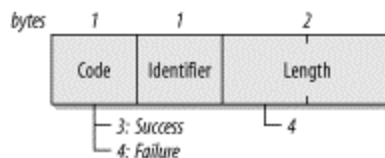
Figure 6-4. EAP Success and Failure frames
